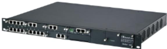
The Mediant 1000 VoIP gateway is a cost-effective, entry level member of the AudioCodes family of SIP gateways. It scales up to 4 E1 / T1 / J1 PSTN trunks in a 1U chassis. Features include NEBS level 3 certified, SIGTRAN backhauling (SS7: M2UA/M3UA,PRI), SS7 peer-to-peer tunneling over IP, G.711, G.723.1, G.726, G.729A codecs, echo cancellation, FAX support, tone generation.
