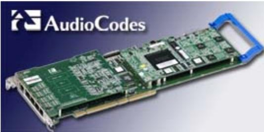
The TP-260 PCI VoIP communications board is a solution for trunking gateways to the PSTN and integrated gateways for IP PBXs and all-in-one communications servers. The TP-260 provides 256 ports for voice, fax or data implementing VoIP media gateway applications.
